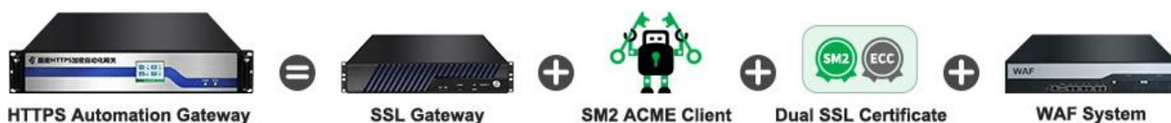
Since the HTTPS encryption and decryption work has been moved from the Web server to the ACME client hardware, the computing power burden of the Web server has been reduced by 20-30%, allowing the Web server to be dedicated to processing user business systems. This function is actually the role of the traditional SSL gateway, which is why ZoTrus Technology named this SM2 ACME client hardware as "HTTPS Automation Gateway", or "ZoTrus Gateway" for short.
